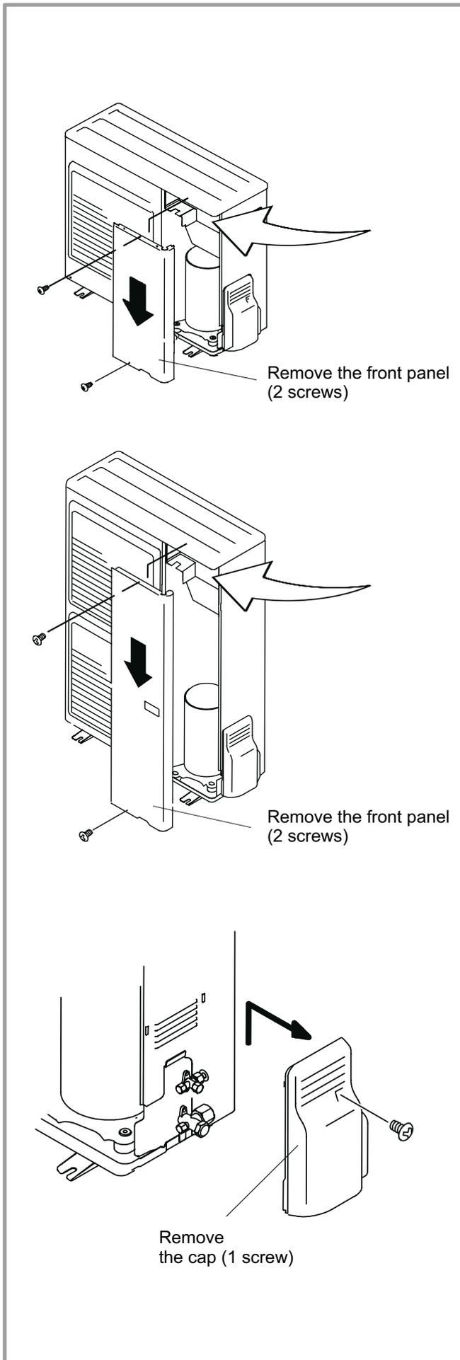
figure 25 - Access to outside unit's terminal block
