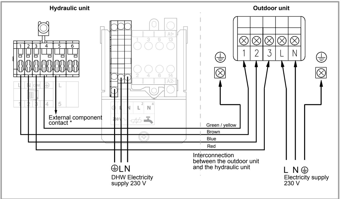
figure 29 - Connection to terminal block and power relays
