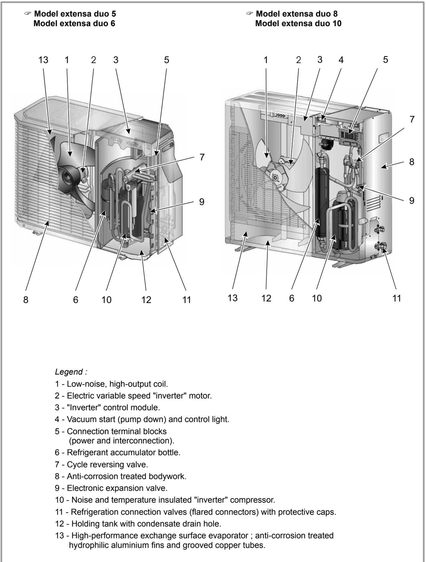
**figure 6 - Outside unit components**
