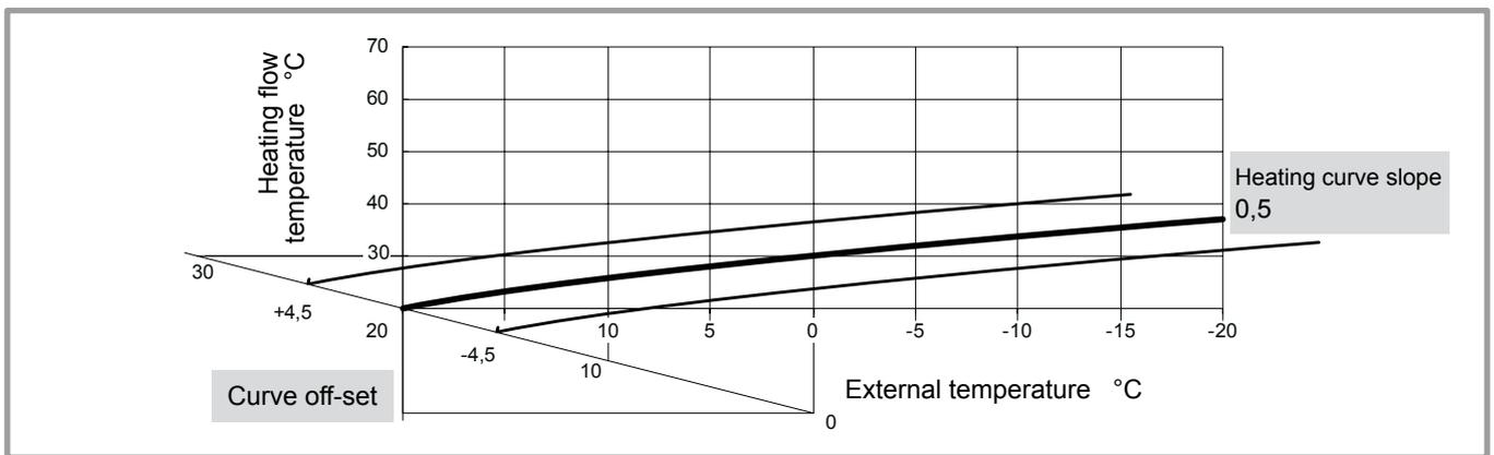
figure 34 - Off-set of the heating curve (line 721)
