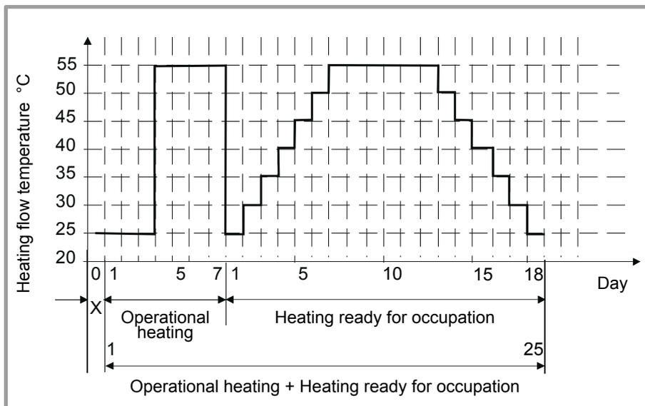
figure 36 - Diagram of the concrete slab drying programmes
