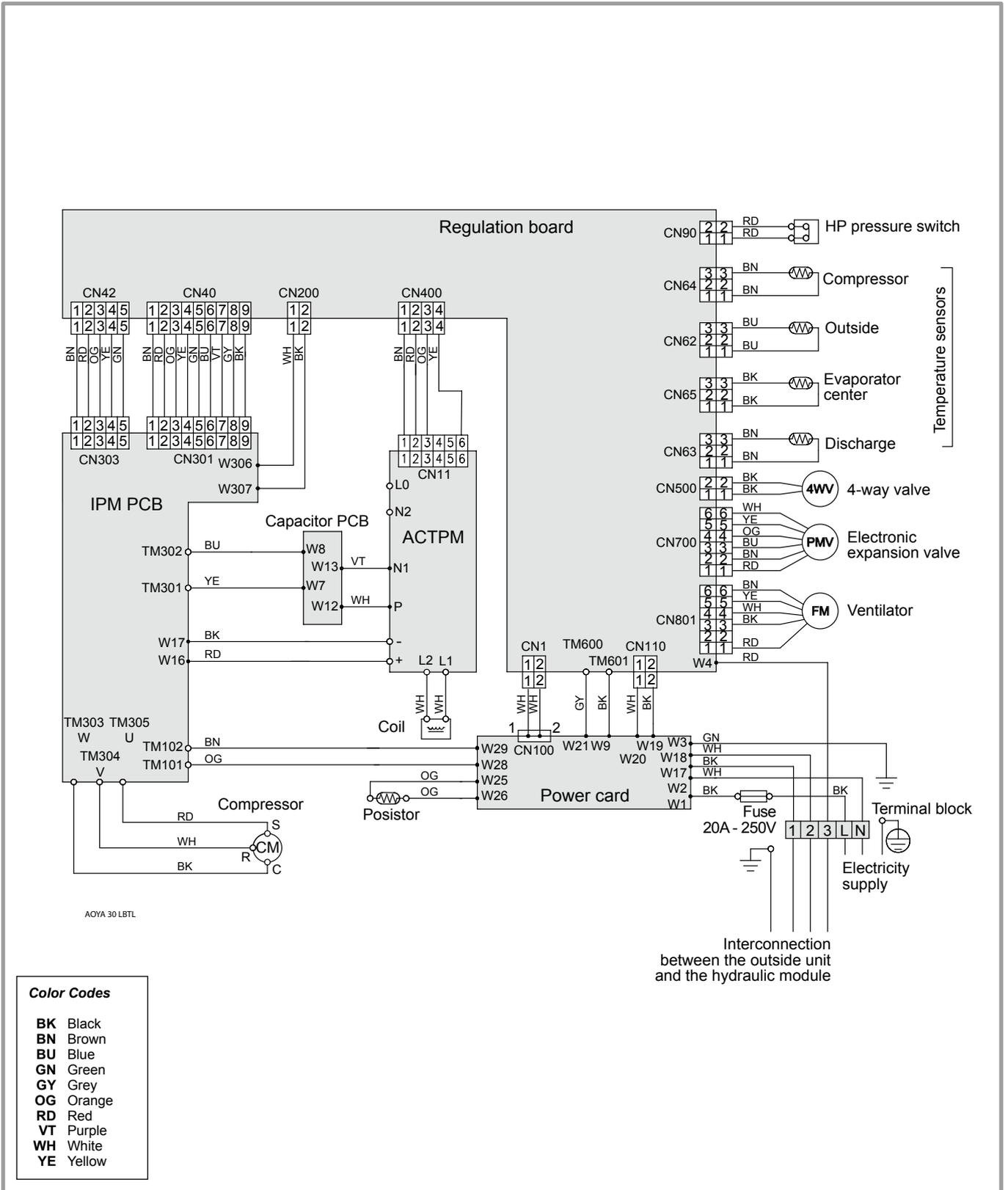
figure 38 - Electrical wiring of outside unit model extensa duo 8 & 10
