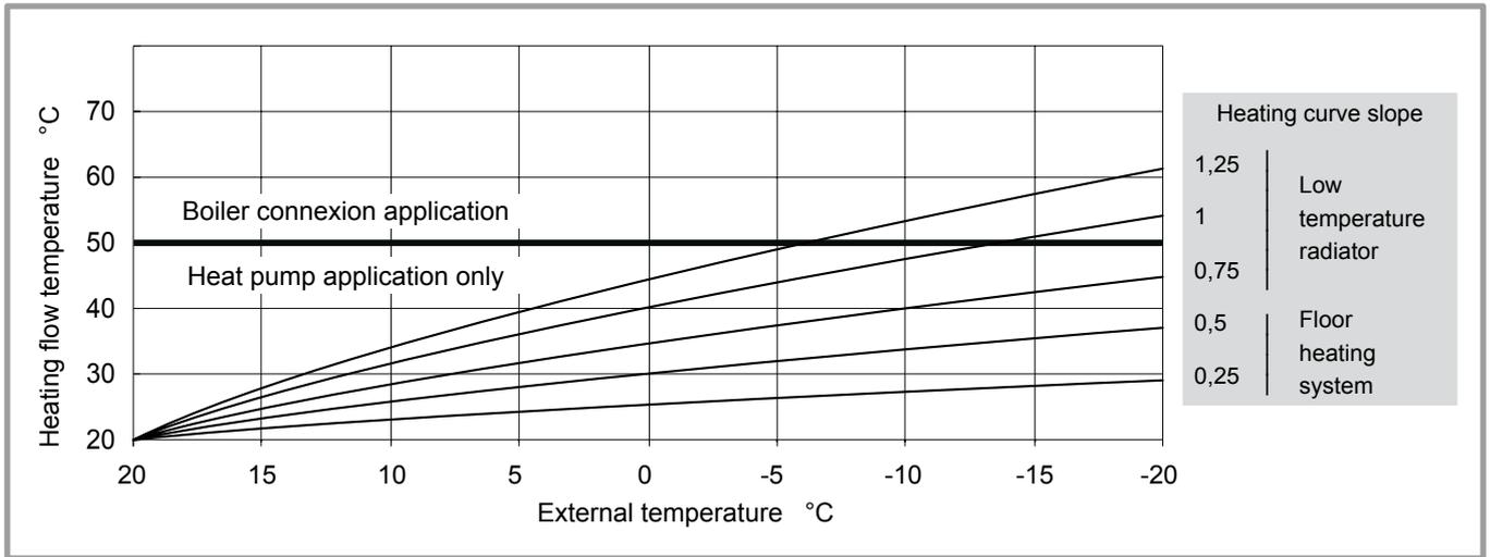
figure 33 - Heating curve slope (line 720)
