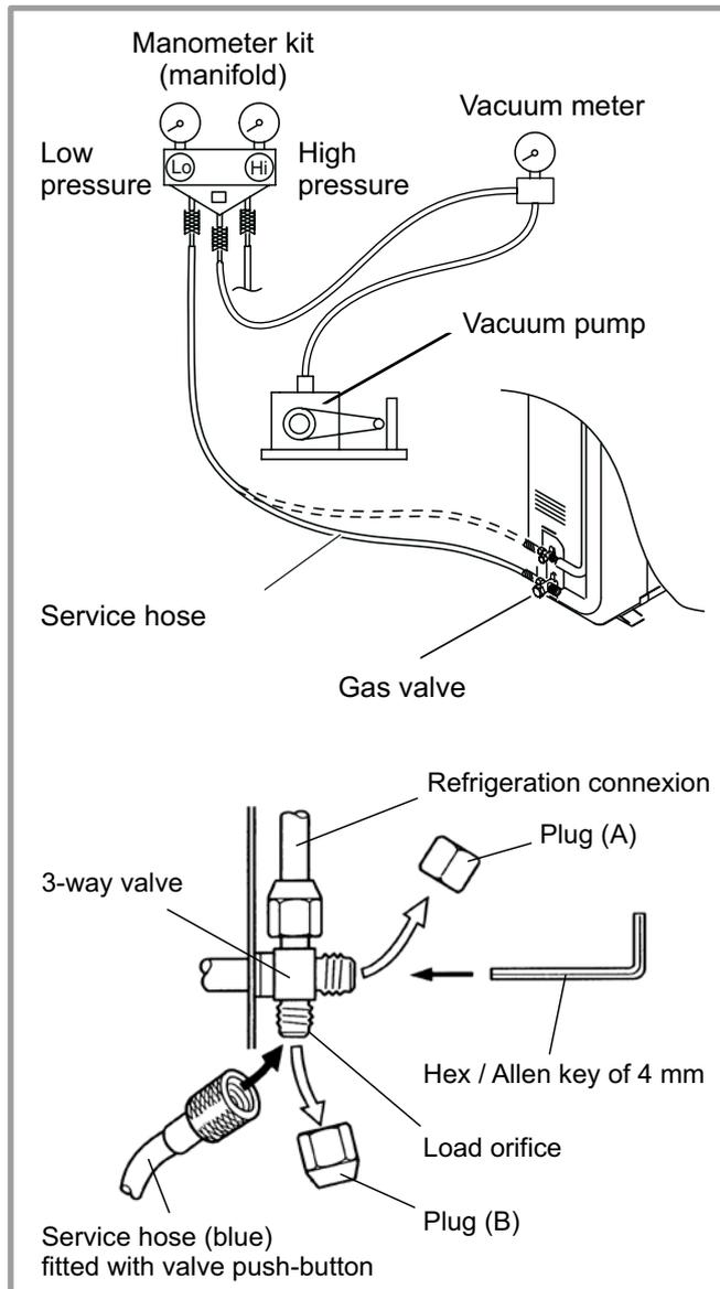
figure 18 - Extraction under vacuum and gassing
