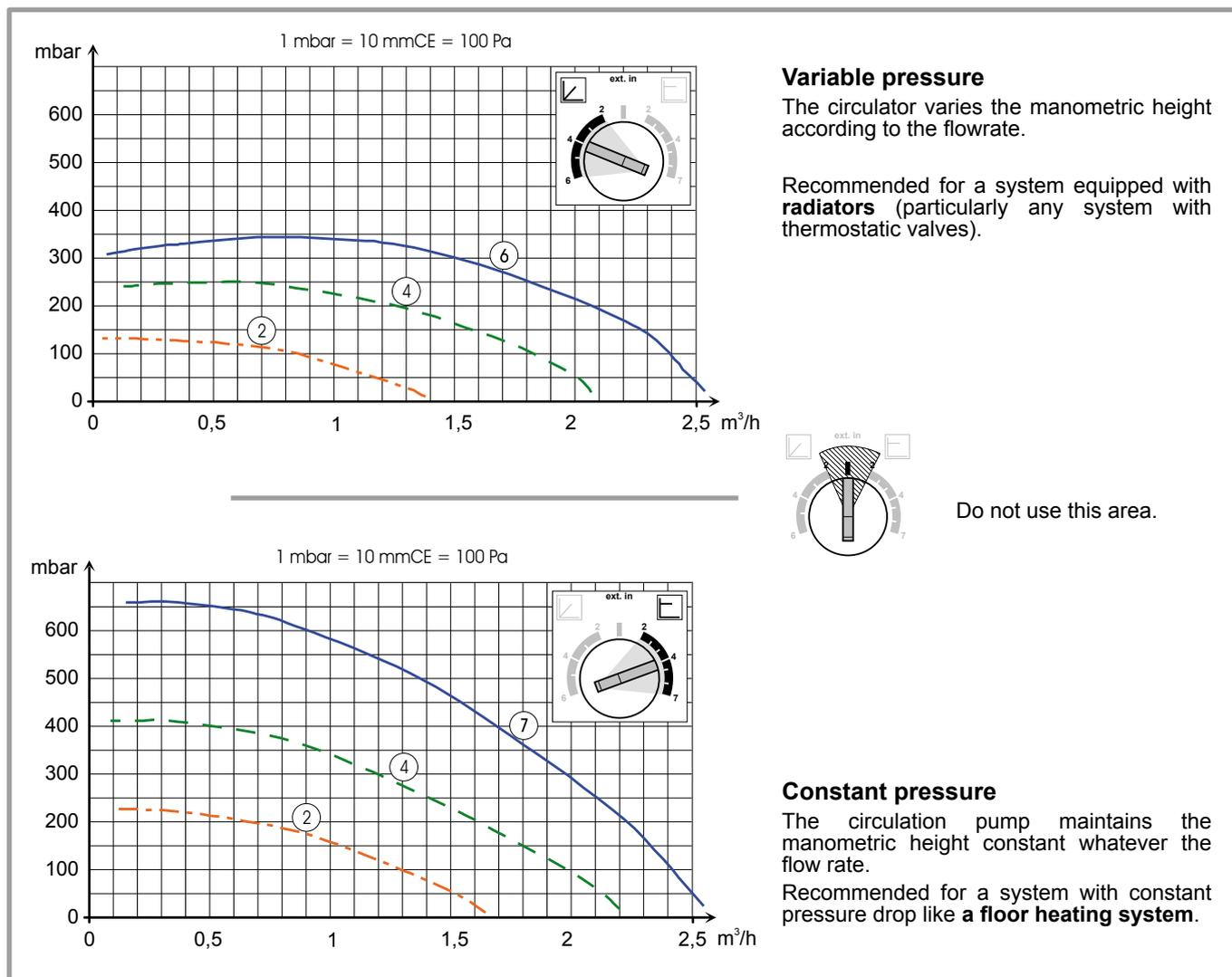
figure 23 - Hydraulic pressures and flow rates available
