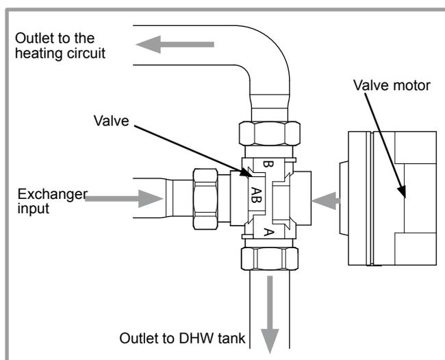
figure 41 - Fitting the distribution valve
