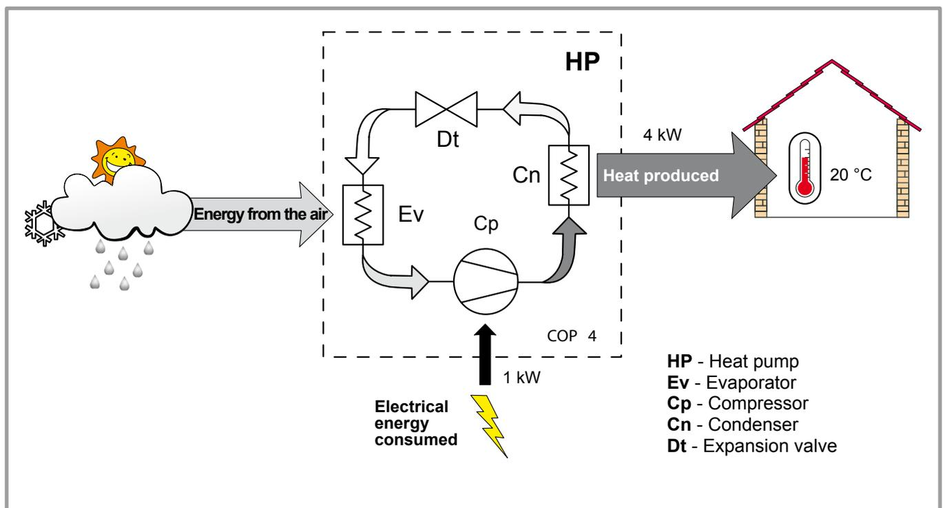
figure 8 - Heat pump operating principle
