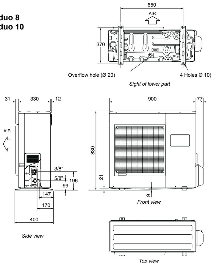
figure 1 - Dimensions in mm
