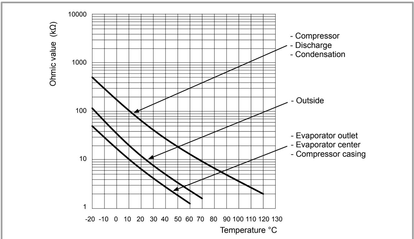
figure 5 - Ohmic values of the sensors (outside unit)
