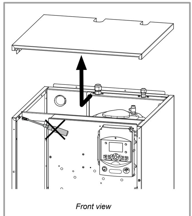
*figure 14 - Removing the cover*
